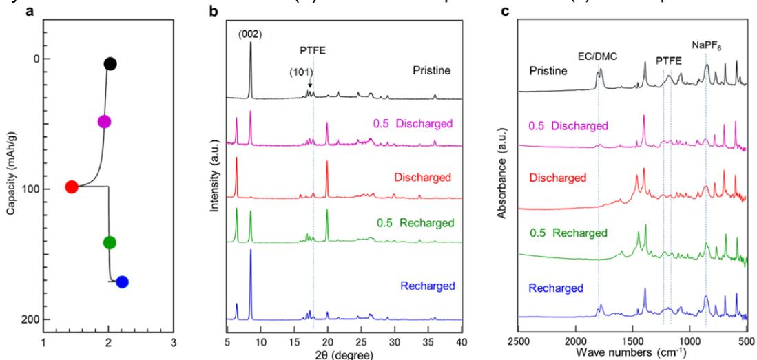
➤ The 002 diffraction peak observed at 8.8° has decreased upon discharging and perfectly disappeared at the end of the discharge cycle and the 002 peak recovered after charging the cell that is indicating the reversibility.
