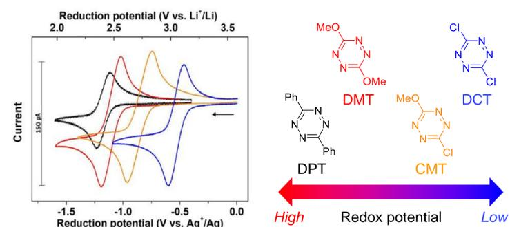
Fig. Cyclic voltammety of s-tetrazines
